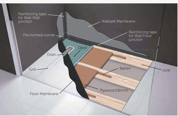
The Drain and Deck are supported by plywood held in place between the floor joists by battens.
